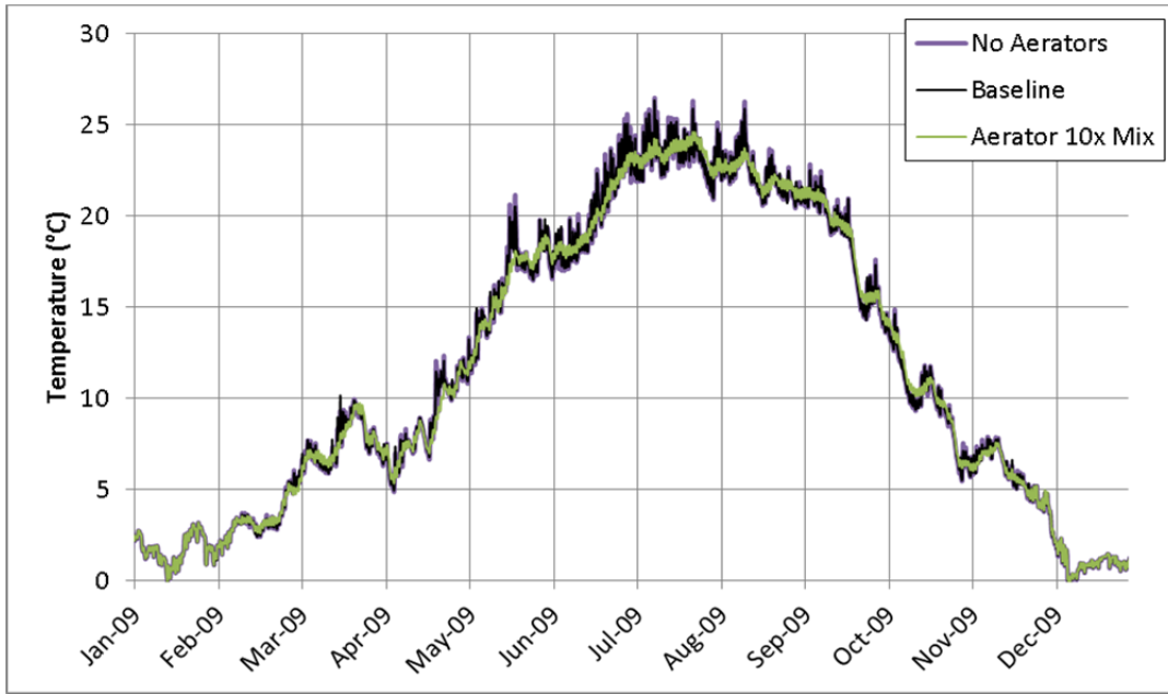
Figure 70. Hourly Simulated Water Temperature at 1 m for Aerator Mixing Simulations, CCR2, 2009
